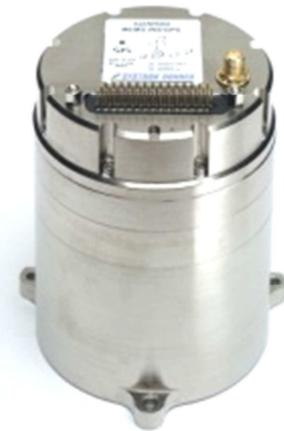
SDI's proprietary Quartz MEMS technology delivers a low total cost of ownership with no wear-out modes or required calibration intervals. The solid state, low noise quartz sensors, robust isolation system and sealed construction provide for excellent environmental performance across temperature, vibration and shock, yielding a reliable 25,000+hr. MTBF, and a 20 year operating and storage life.
